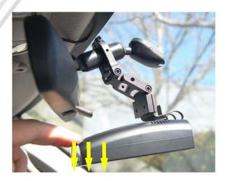
4 - To access the buttons of the RD you will need to gently push downward on the front of the RD with one finger and push the desired button with another finger. Then allow the RD to return to it's original position by gently letting it spring upward. When accessing the buttons, be sure to push the RD downward just enough for your finger to fit between the RD and mirror. Do not push down more than what is needed.
